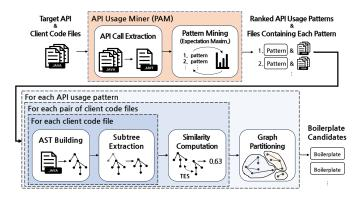
Fig. 1. Overview of the mining process and the steps involved.
