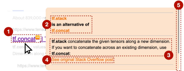
Fig. 2: Overview of our browser plugin: (1) When comparable API methods exist in our labeled dataset, the extension inserts a “vs” icon. The user can hover over it to activate the scrollable tooltip, which displays (2) the pair(s) of comparable API methods, each with links to their reference pages; (3) the relevant sentences for the comparison; (4) a link to the Stack Overflow answer where the sentences were extracted from.
